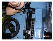
12. 將双腳等高座 C67202F 鎖 上砲塔頭上方孔定位 Feet such as the high seat C67202F lock hole above the turret head positioning
